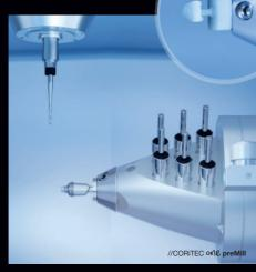
Thanks to the precise rotation axis, CORiTEC preMills and blocks can be machined with optimum quality using the turn-grind process. The automatic 6-fold tool changer ensures full flexibility in material selection.
